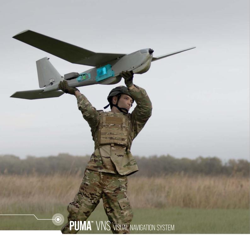
AeroVironment's Puma™ VNS is a visual-based navigation system for Puma AE small unmanned aircraft systems (SUAS). Puma VNS enables GPS-denied navigation across GPS-contested environments. The system performs Visual Inertial Odometry (VIO) through a suite of integrated sensors and an onboard compute module to determine the precise location of the aircraft during flight.
